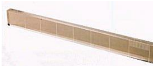
Perspex cutting block for sectioning the Melinex tape into hourly/daily samples
