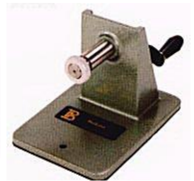
Laboratory stand for coating the recording drum
